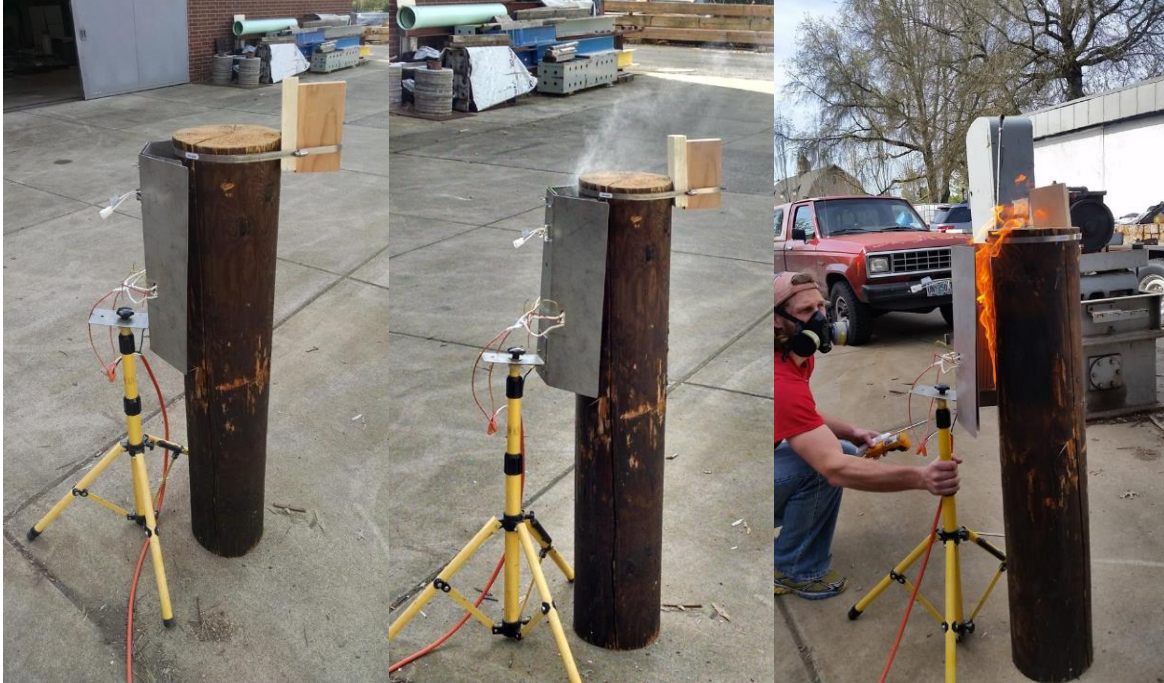
Figure III-11. Example of the fire test apparatus being applied to a pentachlorophenol treated Douglas-fir pole showing initial heating, the beginning of combustion with smoke and finally, the pole on fire.
