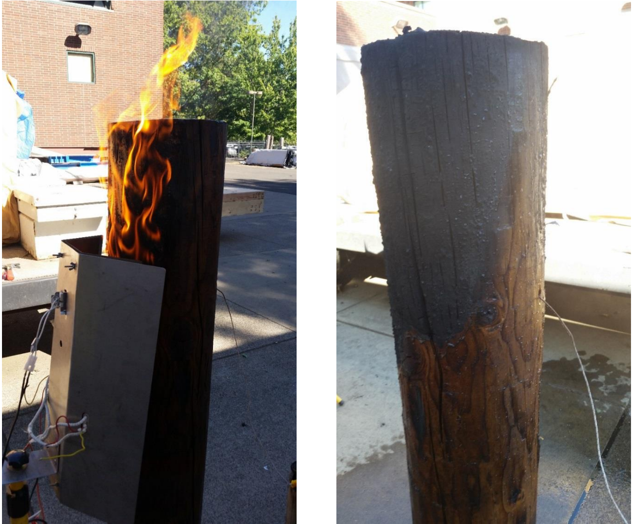
Figure III-16. Example of SunSeeker fire retardant treated pole on fire and pole condition after the fire.
