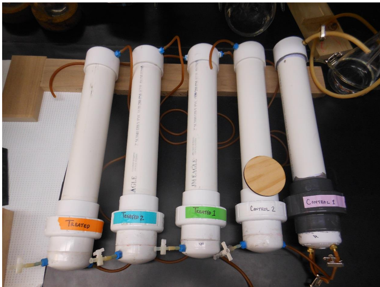
Figure I-19. Photograph of five of the diffusion apparatus used to assess boron movement through non-treated or diesel oil treated Douglas-fir lumber. A wood sample is resting on the fourth chamber to provide a measure of scale.
