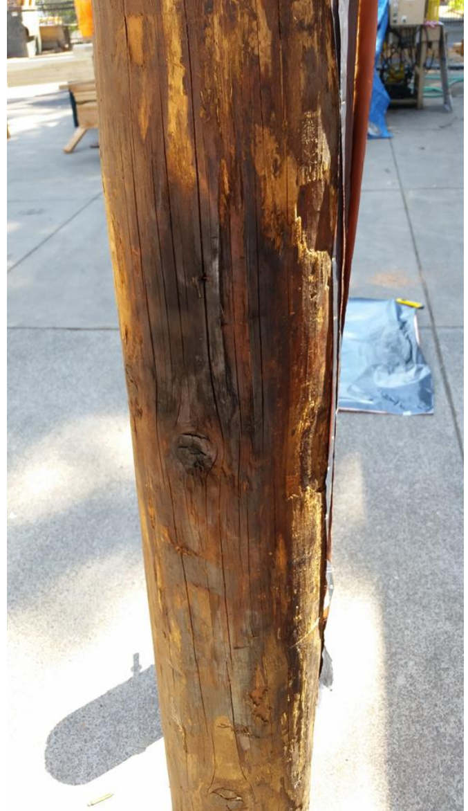
Figure III-15. CopperCare barrier system showing damage to the barrier but only slight charring beneath after the barrier was removed.
