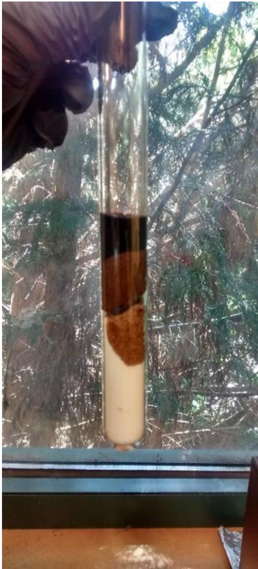
Figure I-9. Examples of tests tubes containing equal amounts of 1% copper naphthenate and dazomet in either granular or powdered form and stored for 24 hours at room temperature.
