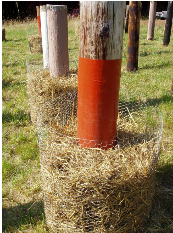
Figure III-8. Example of straw in a wire mesh basket surrounding a pole with a candidate fire retardant wrap.
