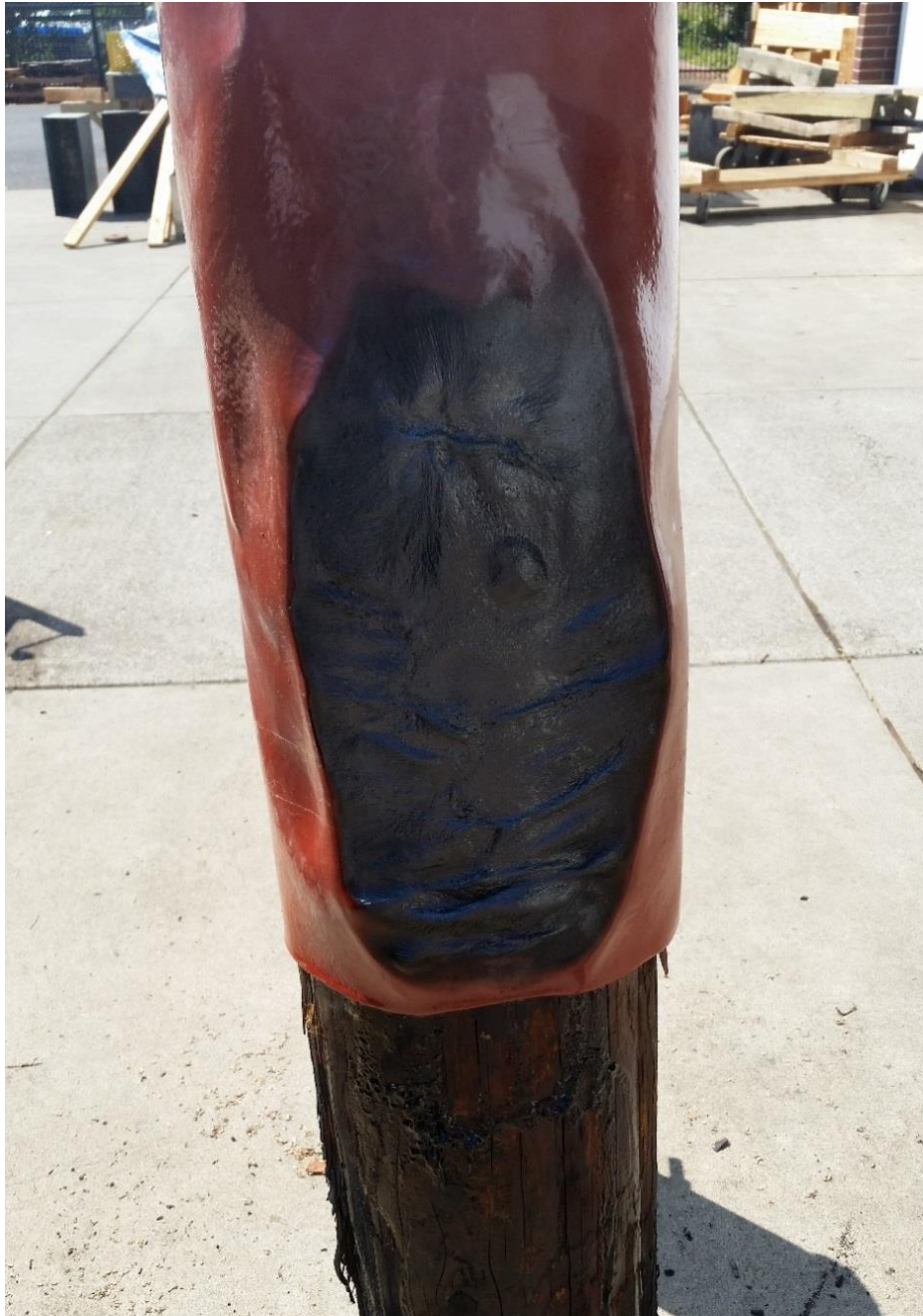
Figure III-14. Brooks fire retardant wrap after test showing charred area of the barrier that protected the pole from fire.
