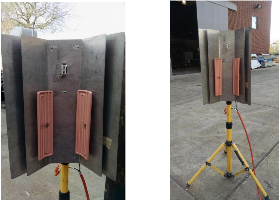
Figure III-10 Example of a potential small scale fire test apparatus showing the heating shield on a tripod and close up of the heating elements.
