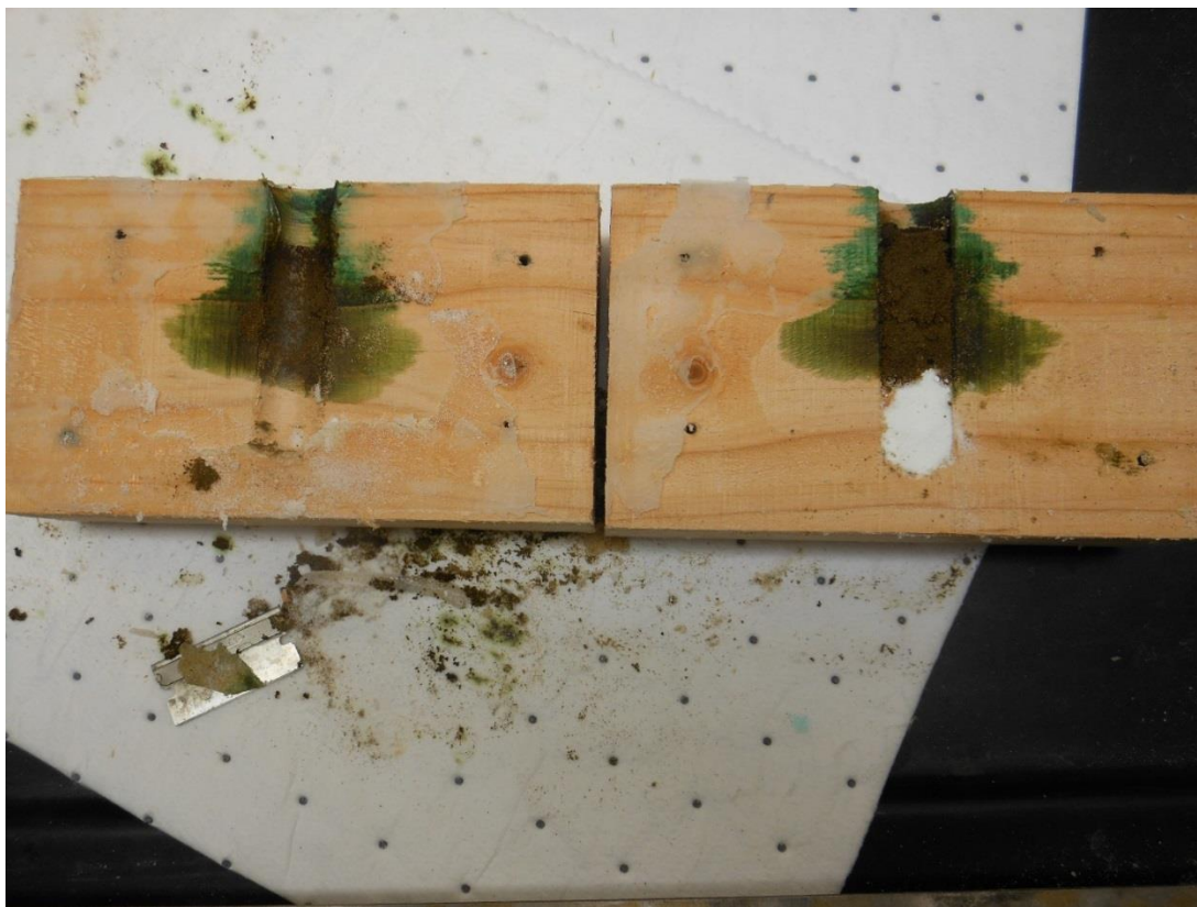
Figure I-11. Example of a 200 mm long block used to assess copper naphthenate distribution patterns in dazomet treatment holes showing copper naphthenate penetration limited to the upper zone of the treatment hole.
