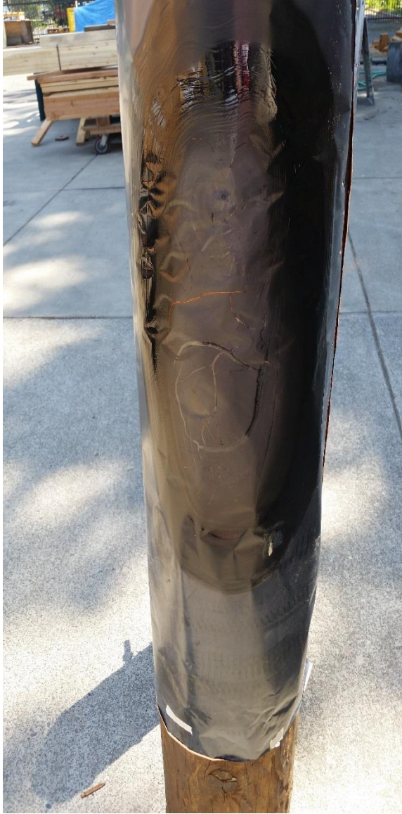
Figure III-15. CopperCare barrier system showing damage to the barrier but only slight charring beneath after the barrier was removed.
