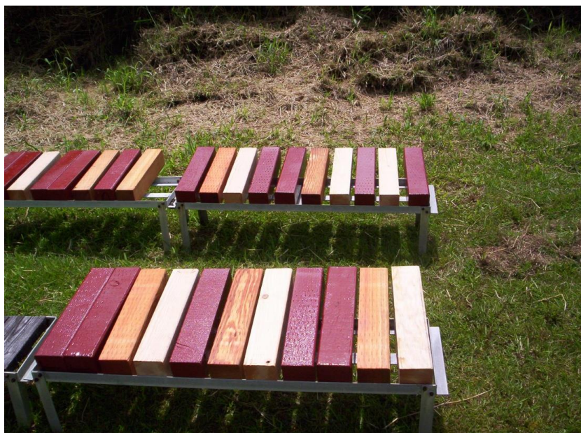
Figure III-1. Polyurea coated and non-coated samples shortly after exposure in Hilo Hawaii.
