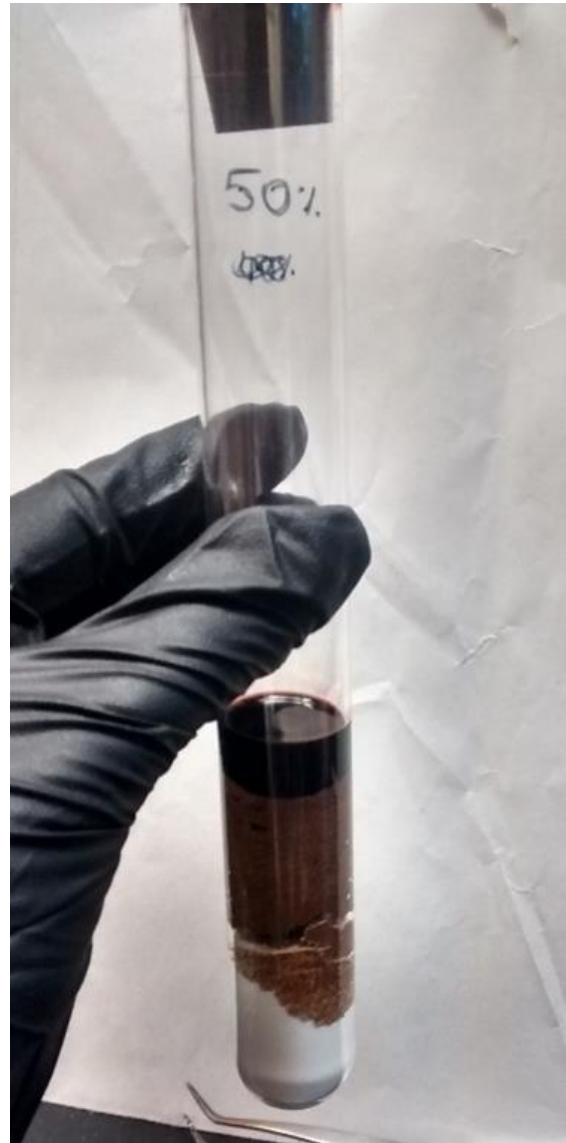
Figure I-9. Examples of tests tubes containing equal amounts of 1% copper naphthenate and dazomet in either granular or powdered form and stored for 24 hours at room temperature.
