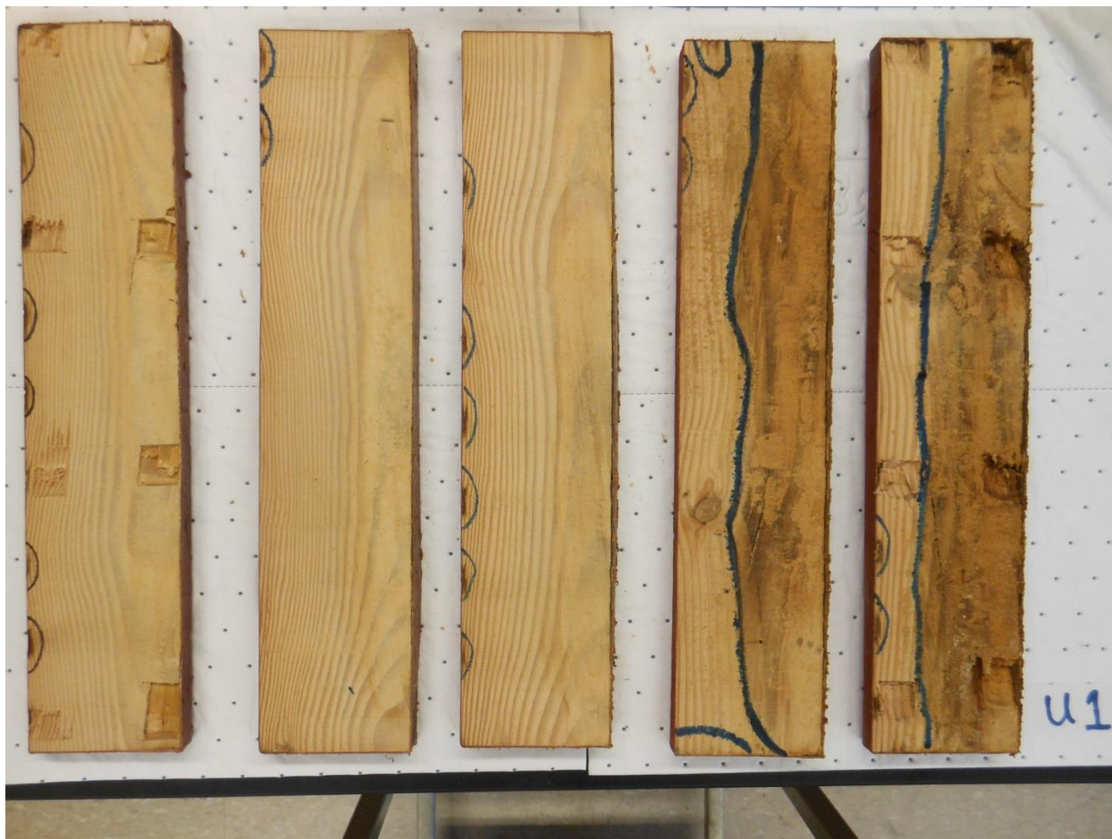
Figure III-5. Example of the interior of a coated, untreated Douglas-fir section after 6 years of aboveground exposure in Hilo, Hawaii.
