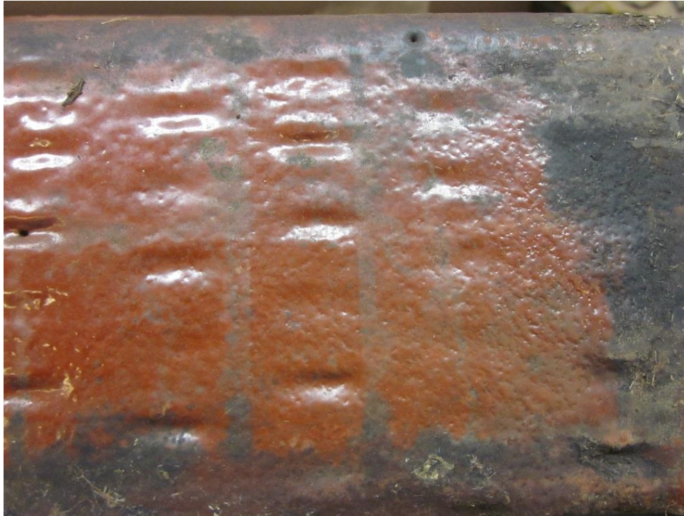
Figure III-2. Example of lower, non-UV exposed surface of a coated, penta-treated section showing evidence of oil migration towards the coating surface after 6 years of exposure in Hilo, Hawaii.
