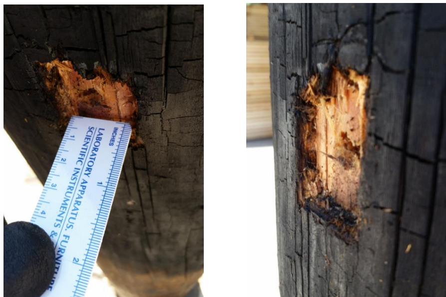
Figure III-12. Example of char scrapped from the pole surface to reveal non-burned wood beneath.
