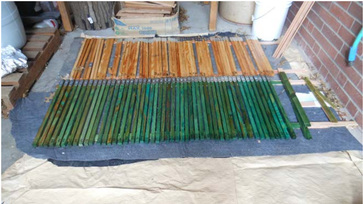
Figure III-8. Stakes drying under cover after treatment with copper naphthenate (bottom) or penta (top).
