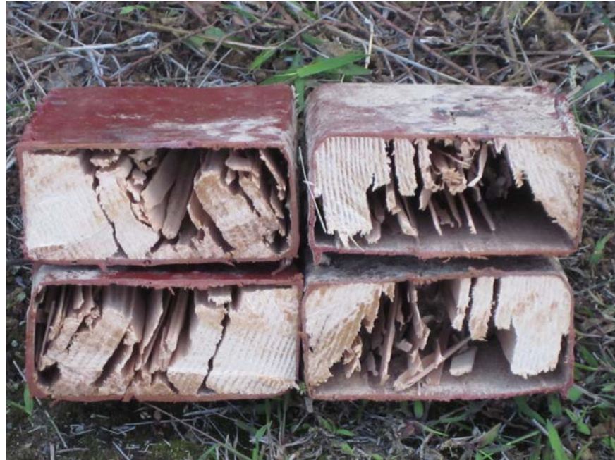
Figure III-3. Cross sections cut through polyurea coated sections of non-treated Douglas-fir (left) and Douglas-fir dip-diffusion treated with borates prior to coating (right) after 1 year of exposure to Formosan termite attack.
