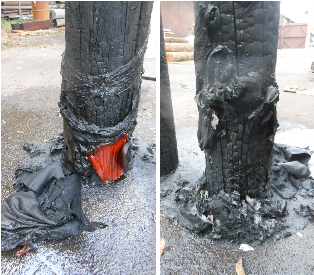
Figure III-26. Polyurea wrapped pole shortly after testing and then 20 minutes after the flame was removed showing extensive charring and loss of the coating.
