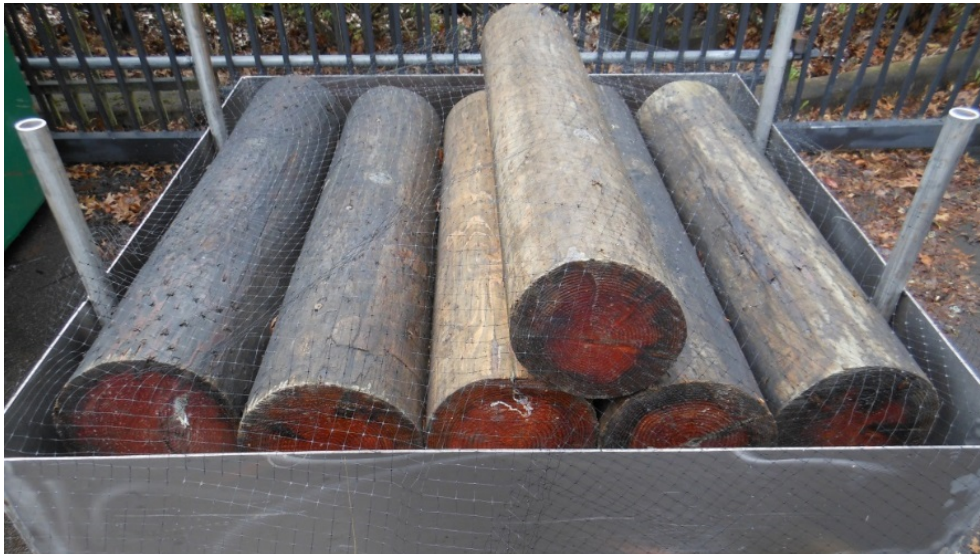
Figure VI-1. The six-pole configuration evaluated in our small scale preservative migration chamber.
