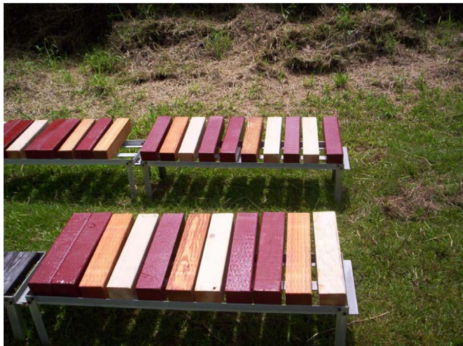
Figure III-4. Example of Douglas-fir crossarms with and without polyurea coating immediately after exposure near Hilo, Hawaii.
