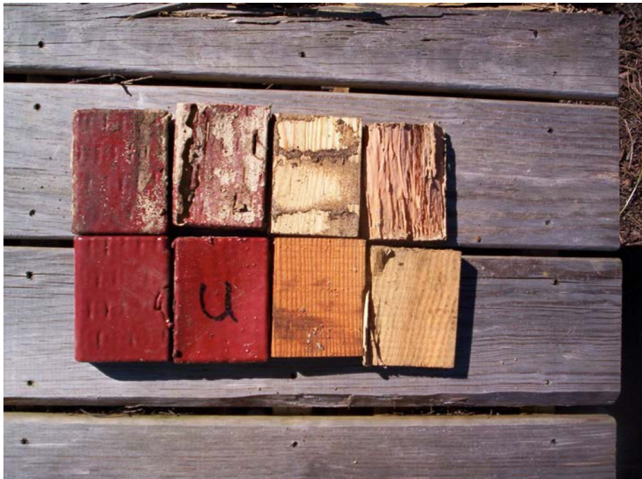
Figure III-2. Examples of the undersides (top) and upper surfaces of coated and non-coated Douglas-fir lumber with and without penta treatment. From the left, the samples are coated/penta-treated, coated/non-treated, non-coated/penta-treated and non-coated/non-treated after 6 months of exposure to Formosan termite attack.
