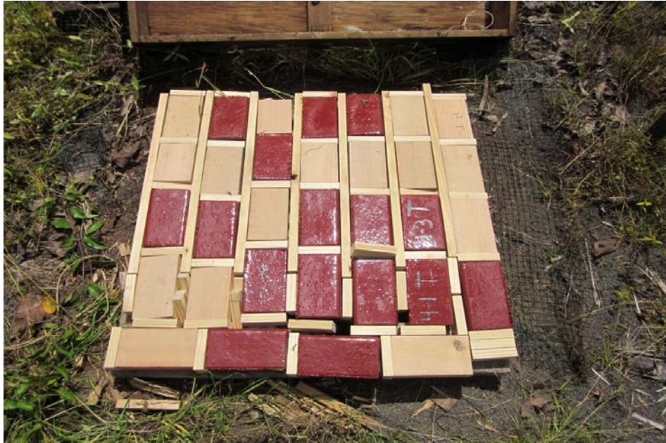
Figure III-1. Example of a termite array containing coated and non-coated Douglas-fir lumber sections at the time of exposure.
