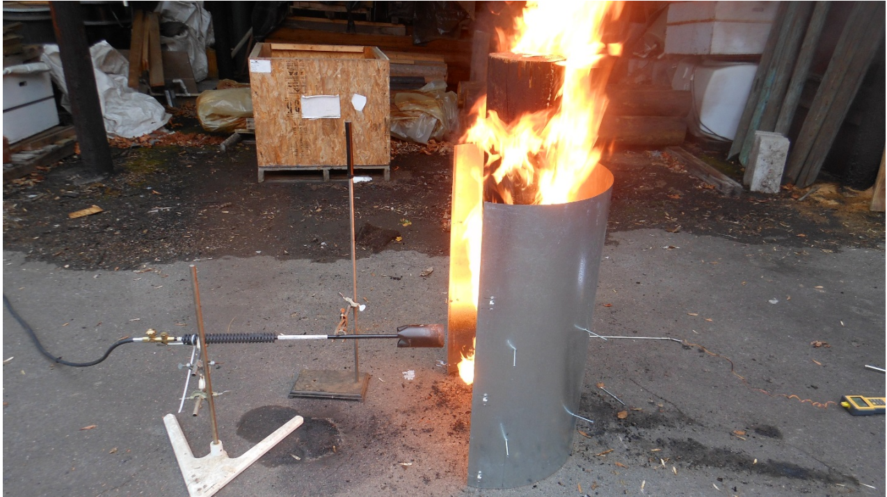
Figure III-23. Non-coated pole undergoing flame test.
