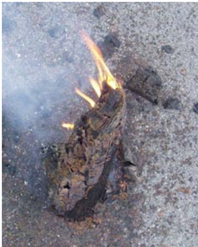
Figure III-21. Example of a copper naphthenate treated Douglas-fir pole subjected to burning that completely burned.
