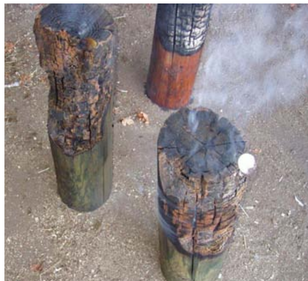
Figure III-20. Examples of copper naphthenate treated Douglas-fir pole sections after a burn exposure test.
