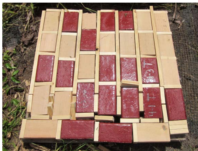
Figure III-15. Example of a termite array containing coated and non-coated Douglas-fir lumber sections at the time of exposure.
