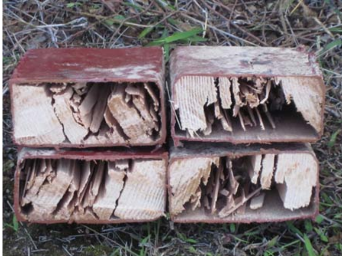
Figure III-17. Cross sections cut through polyurea coated sections of non-treated Douglas-fir (left) and Douglas-fir dip-diffusion treated with borates prior to coating (right) after 1 year of exposure to Formosan termite attack.
