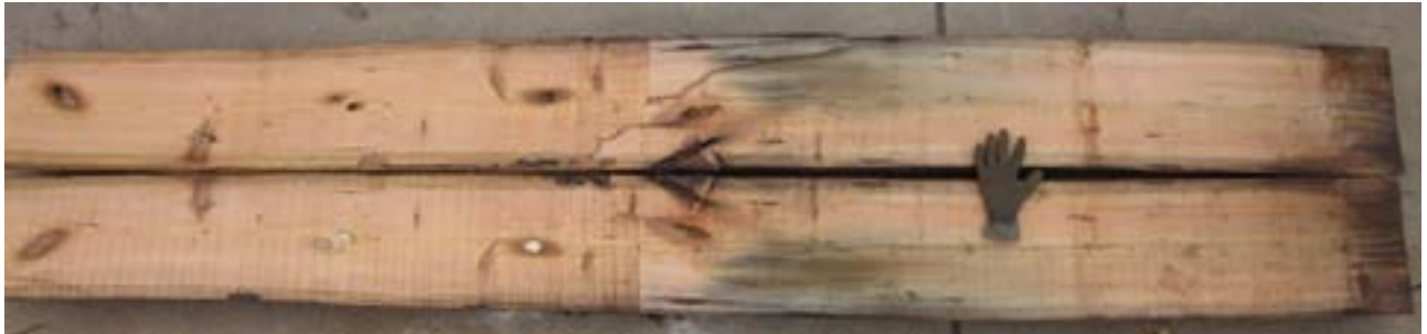
Figure III-29 Longitudinal section cut through the butt of a pole showing preservative end-penetration (left) and the sloping hole from a inspection/remedial treatment site, but no evidence of internal decay.
