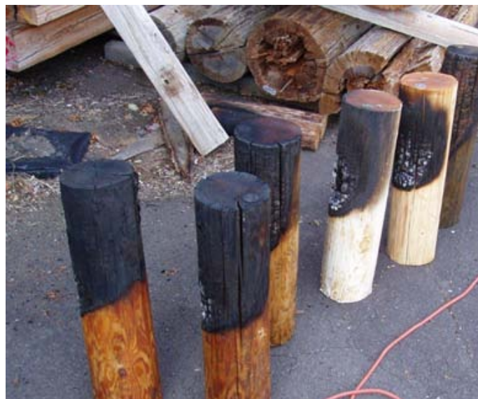
Figure III-19. Examples of penta (left) and non-treated (right) Douglas-fir pole sections after burning showing charring.
