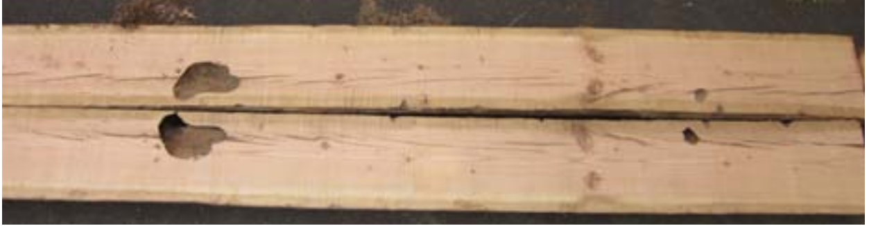
Figure III-28 Longitudinal cross section through a two part of a pole showing clear wood near the butt (top section) and extensive internal decay near the top (bottom section).
