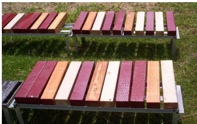
Figure III-13. Examples of Douglas-fir crossarm sections with and without polyurea coating immediately after exposure near Hilo, Hawaii.
