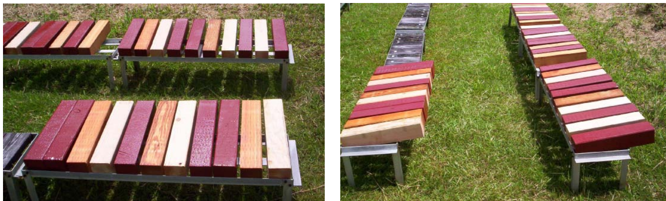
Figure III-2. Examples of Douglas-fir crossarm sections with and without polyurea coating immediately after exposure near Hilo, Hawaii.
