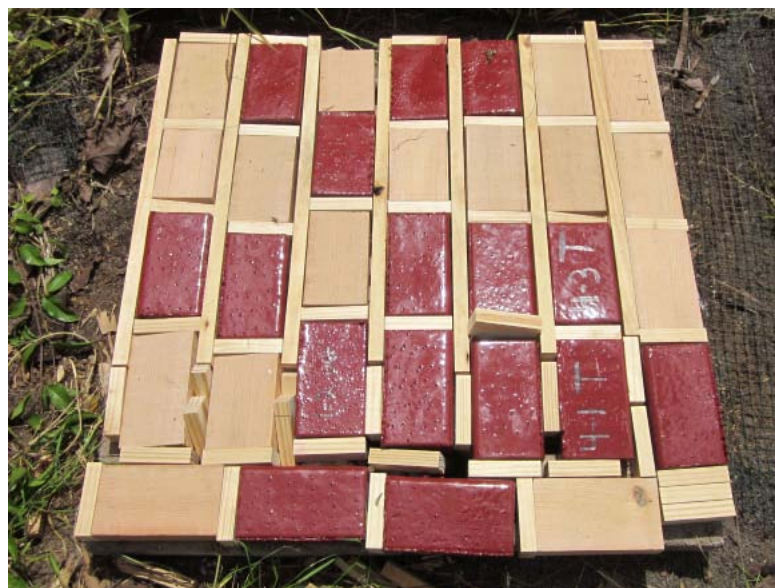
Figure III-5. Example of a termite array containing coated and non-coated Douglas-fir lumber sections at the time of exposure.
