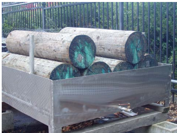
Figure VI-1 Poles in the rainfall runoff collection tank.
