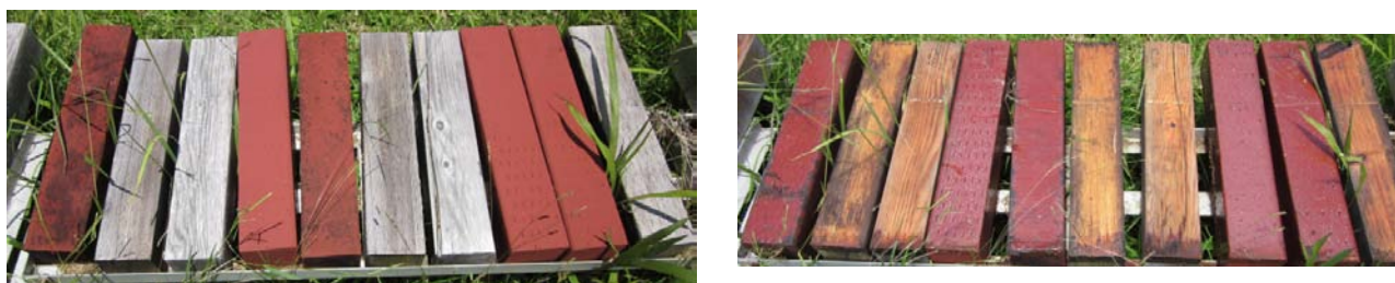
Figure III-4. Examples of the upper surfaces (UV exposed, left) and undersides (right) of coated and non-coated Douglas-fir crossarm sections 18 months after installation near Hilo, Hawaii.
