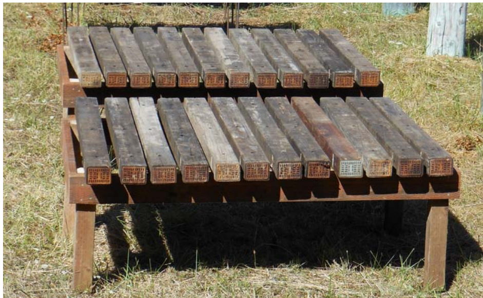
Figure III-1. Douglas-fir crossarms with end plates on one end and no plate on the other on racks above the ground at the Peavy Arboretum test site.
