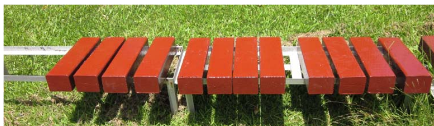
Figure III-3. Polyurea coated Douglas-fir arm sections exposed in June 2011.
