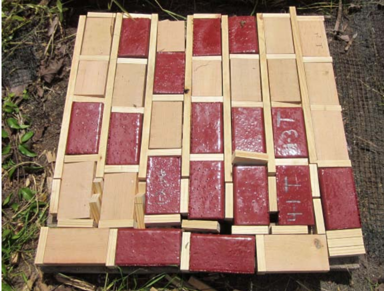
Figure III-3. Example of a termite array containing non-coated and polyurea coated Douglas-fir lumber sections at the time of exposure.
