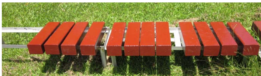
Figure III-2. Polyurea coated Douglas-fir crossarm sections exposed in June 2011.
