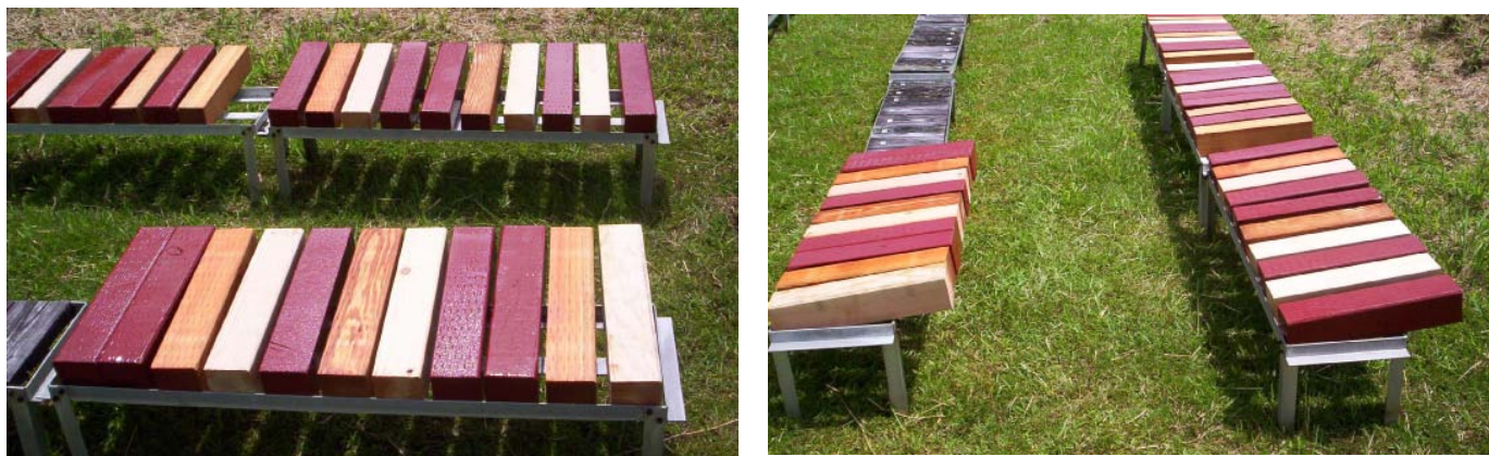
Figure III-1. Examples of Douglas-fir crossarm sections with and without polyurea coating immediately after exposure near Hilo, Hawaii.
