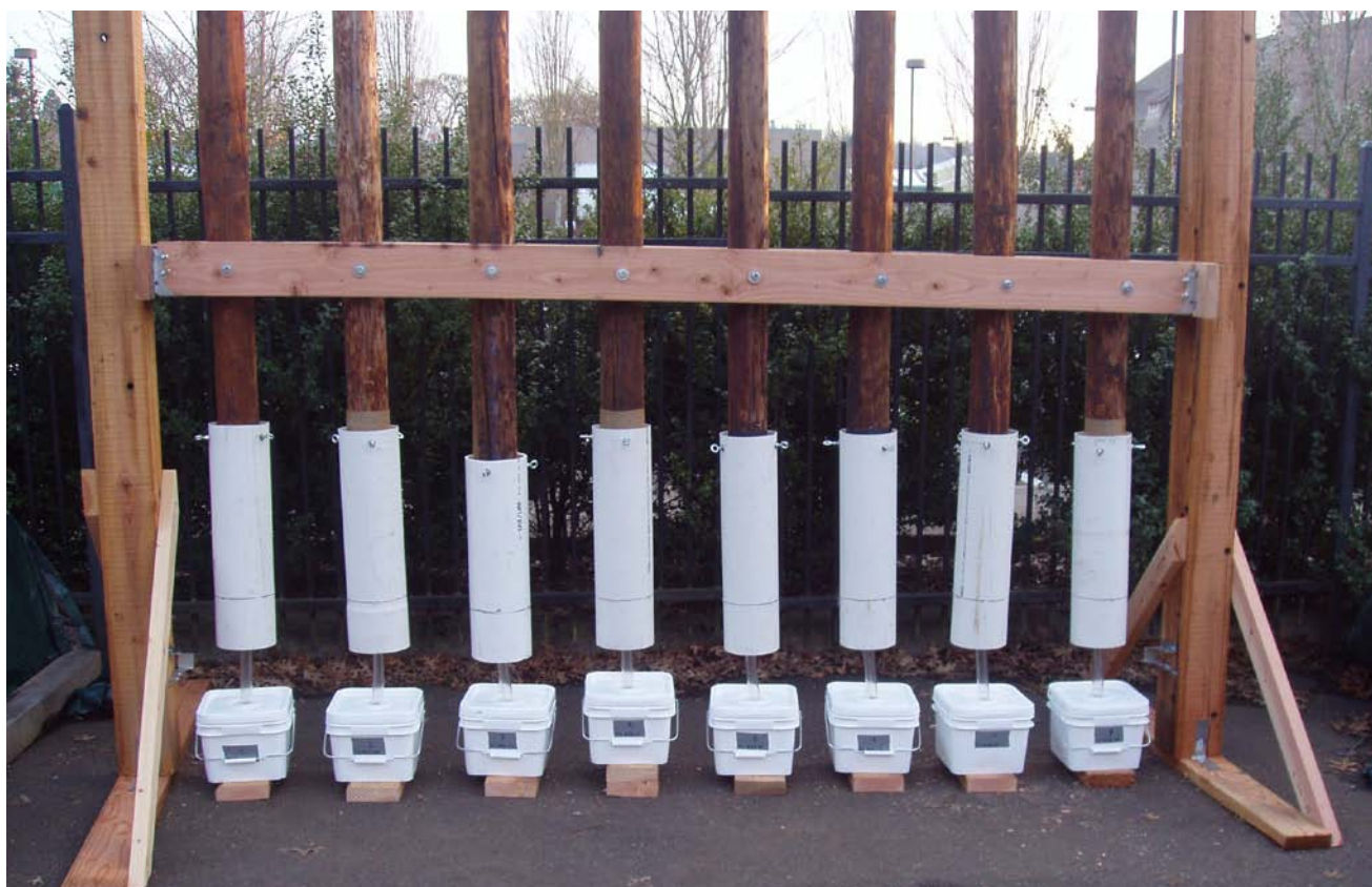
Figure IV-1. Post sections treated with groundline paste showing the plastic containment tubes and the containers used to capture runoff.
