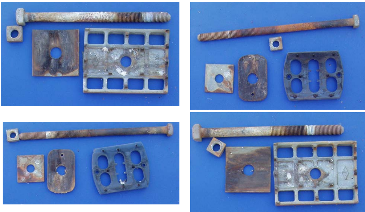
Figure II-3. Condition of nuts, bolts and gain plates removed from field drilled bolts holes 32 years after treatment of the exposed non-treated wood with Boracol prior to bolt insertion.
