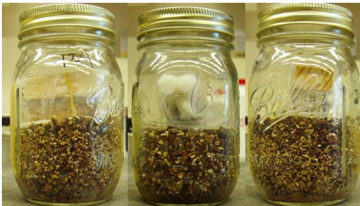
Figure V-4. Decay assemblies in glass jars used to assess the potential for P. placenta to move from the inoculated Douglas-fir heartwood to copper naphthenate treated Douglas-fir sapwood
