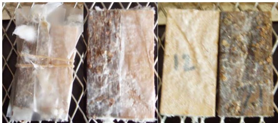
Figure V-3. Examples of Douglas-fir block assemblies used to evaluate the potential for P. placenta to move from the heartwood to copper naphthenate treated sapwood where A) 2 blocks wrapped in plastic, B) the blocks outside the wrap and C) the sapwood/heartwood (left/right) blocks side by side.
