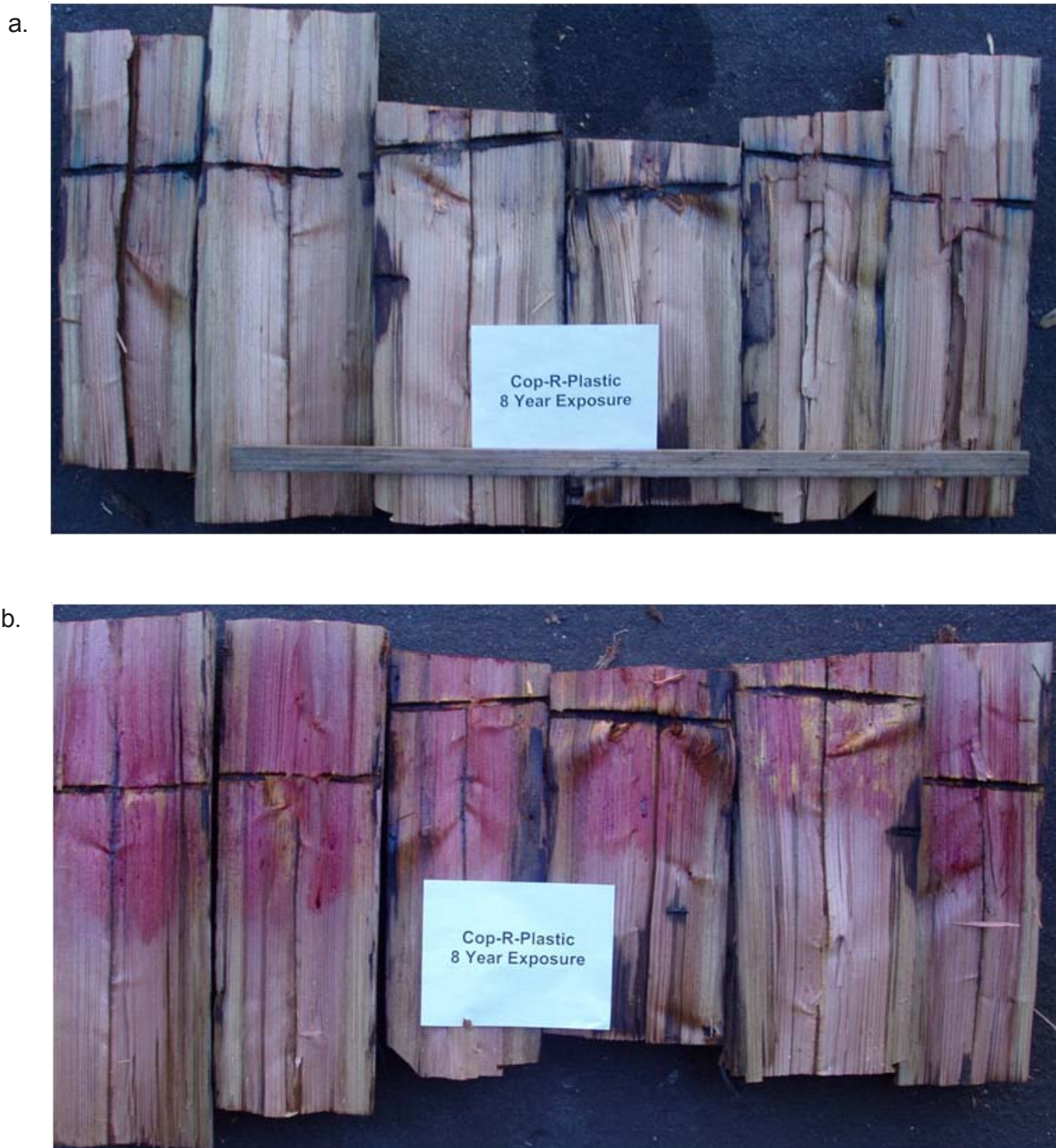
Figure II-1. Degree of a) copper and b) fluoride movement away from the sites in Douglas-fir pole stubs where Cop-R-Plastic coated galvanized threaded rods were installed 8 years earlier.
