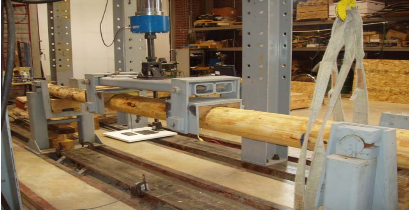
Figure III-1. Photograph showing a pole in the test set-up.
