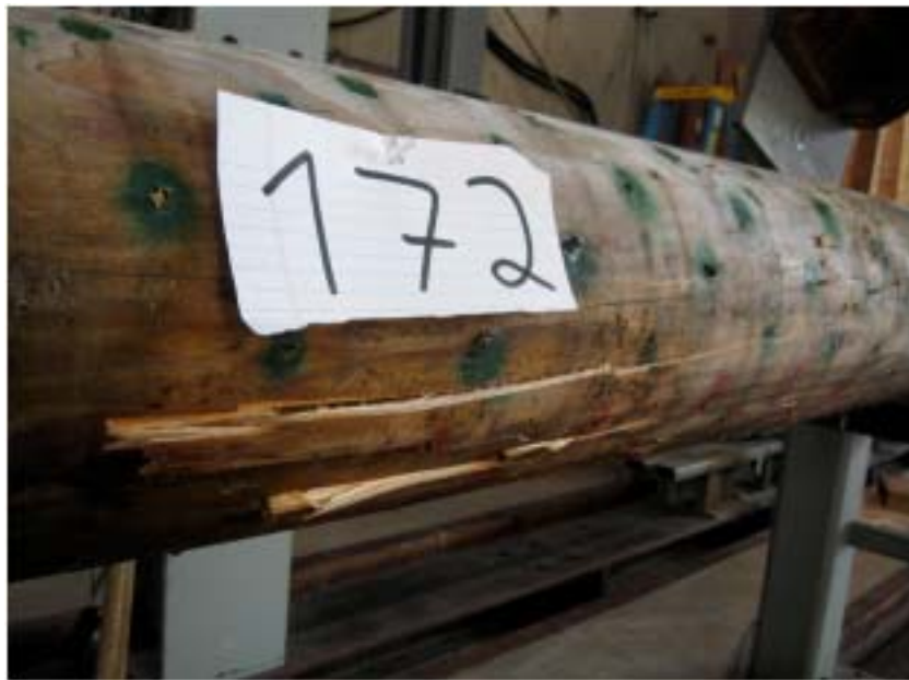
Figure III-2. Example of a typical tension failure on a through-bored Douglas-fir pole.
