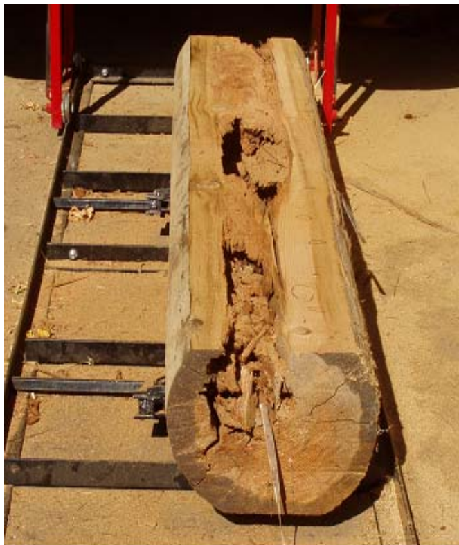
Figure III-13. Example of a section through a Douglas-fir pole showing an association between golden buprestid galleries (circled areas) and dampwood termites.
