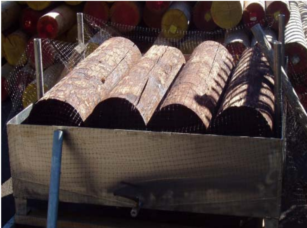
Figure VI-1 (cont.). Photo showing the two six-pole configurations a) configuration 1, b) configuration 2, and c) the four-pole configuration evaluated in our small scale preservative migration chamber.
