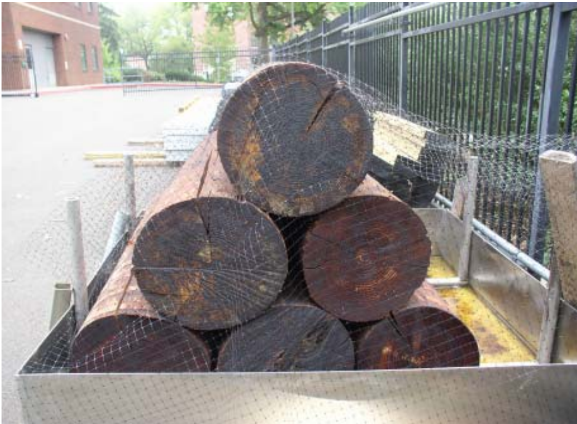
Figure VI-1. Photo showing the two six-pole configurations a) configuration 1, b) configuration 2, and c) the four-pole configuration evaluated in our small scale preservative migration chamber.
