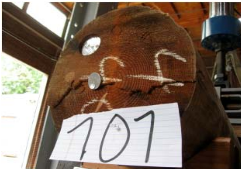
Figure III-3. Example of a shear failure on a deep incised Douglas-fir pole.
