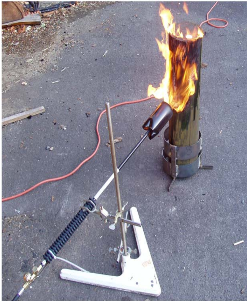
Figure III-8. Apparatus used to evaluate fire resistance of post sections treated with pentachlorophenol in various P9 Type A solvents.
