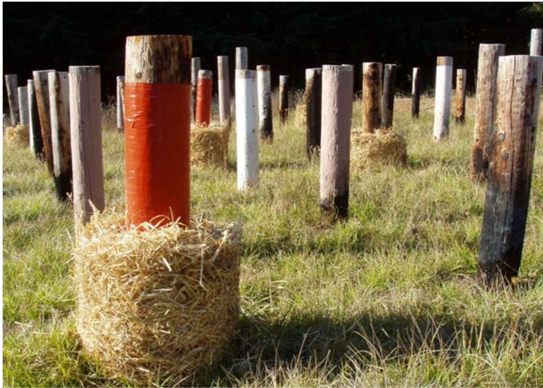
Figure III-6. Example of a pole section with straw in cage prior to ignition.
