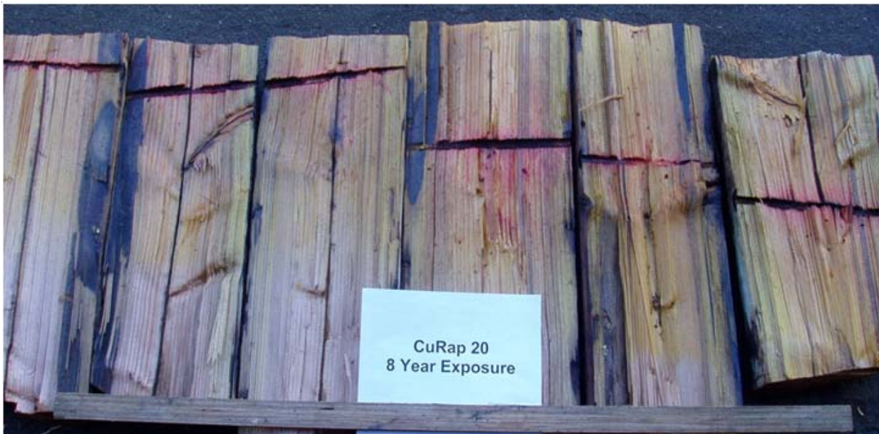
Figure II-2. Degree of a) copper and b) boron movement away from the sites in Douglas-fir pole stubs where CuRap 20 coated galvanized threaded rods were installed 8 years earlier.
