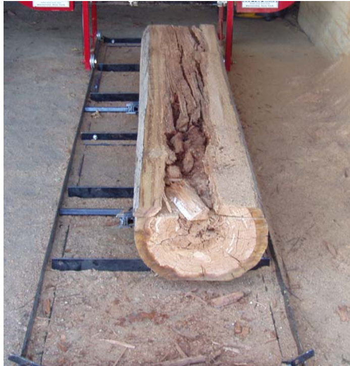
Figure III-4. Example of a section through a Douglas-fir pole showing internal decay.
