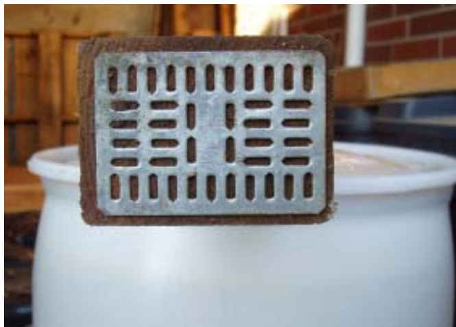
Figure III-2. Example of an end-plate on a penta treated Douglas-fir cross arm.
