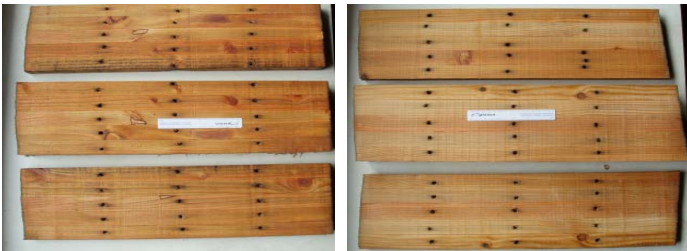
Figure III-14. Preservative penetration in laminated timber sections through-bored at 150 mm intervals and pressure treated with pentachlorophenol.
