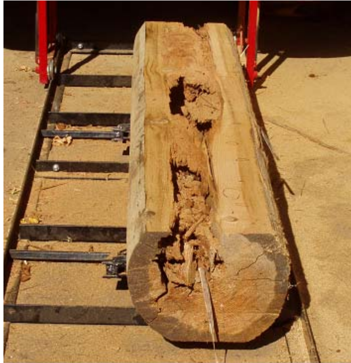
Figure III-6. Example of a section through a Douglas-fir pole showing an association between golden buprestid galleries (circled areas) and dampwood termites.
