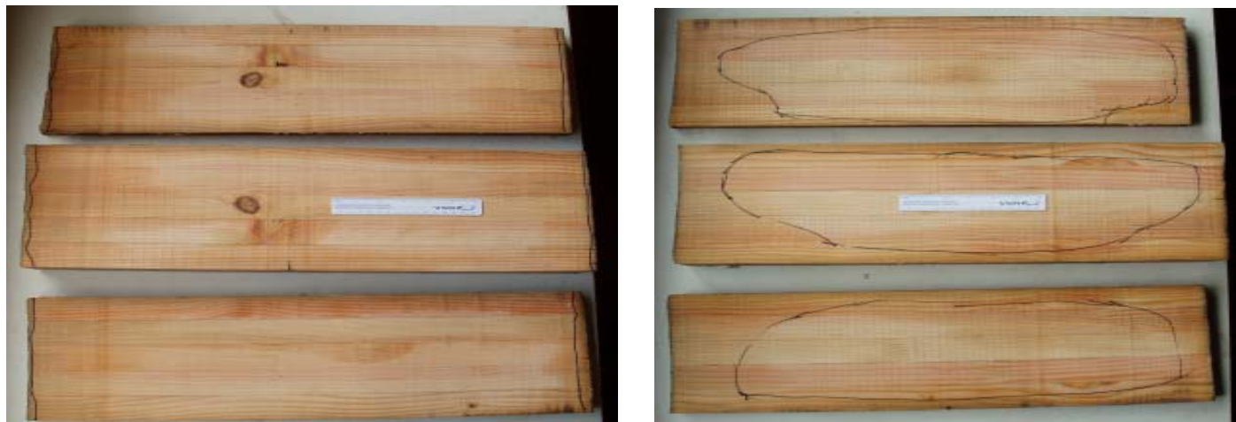
Figure III-10. Preservative penetration in laminated timber sections without through-boring and pressure treated with pentachlorophenol.
