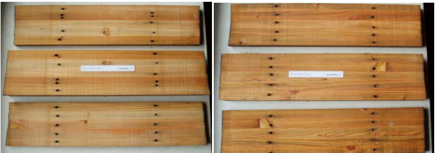
Figure III-12. Preservative penetration in laminated timber sections through-bored at 300 mm intervals and pressure treated with pentachlorophenol.
