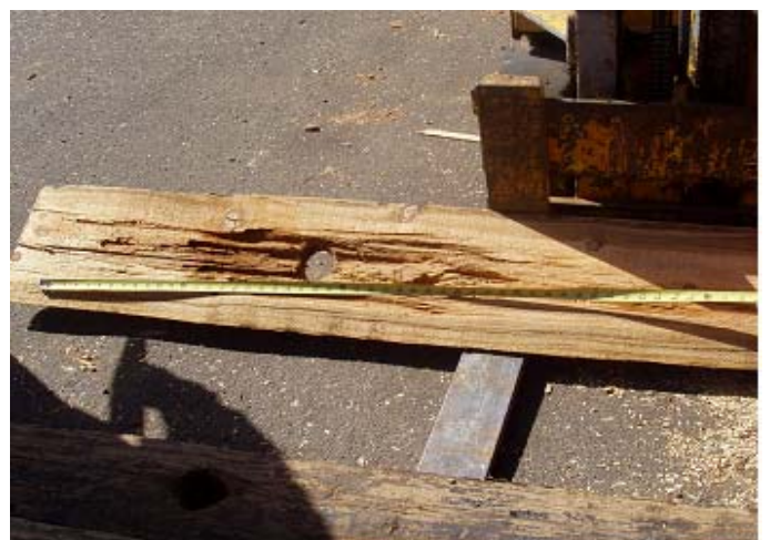
Figure III-5. Example of sections through a Douglas-fir pole showing a woodpecker hole on the surface and the extent of the internal damage associated with the hole.
