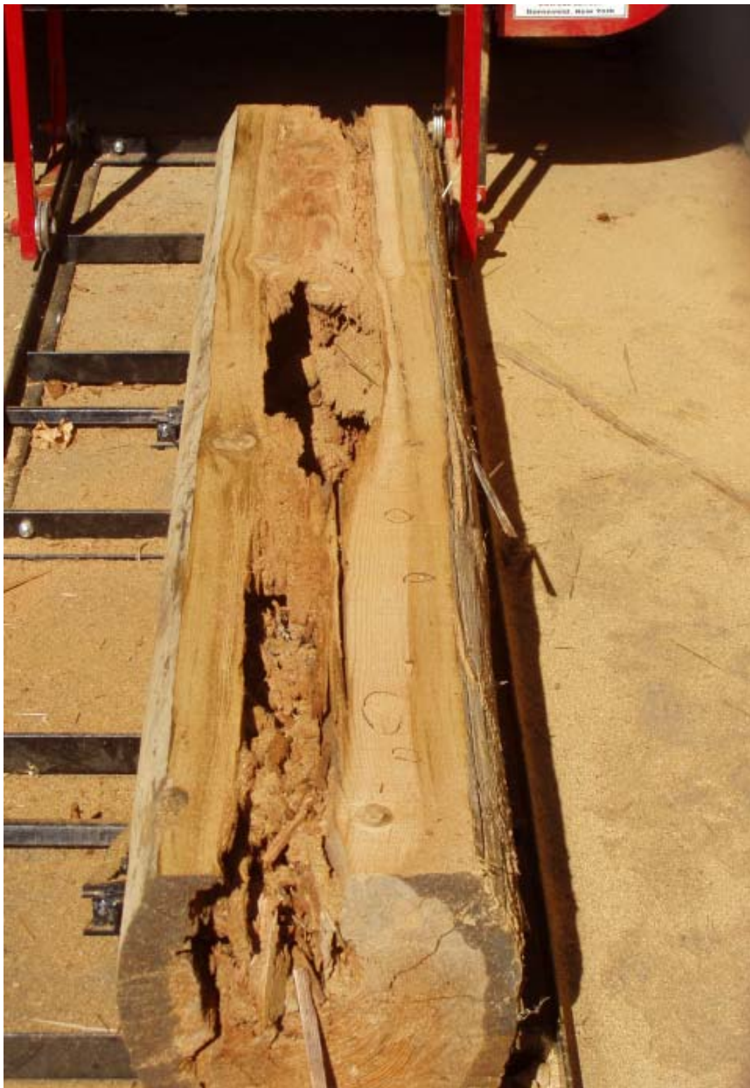
Figure III-5. Example of a section through a Douglas-fir pole showing an association between golden buprestid galleries (circled areas) and dampwood termites.
