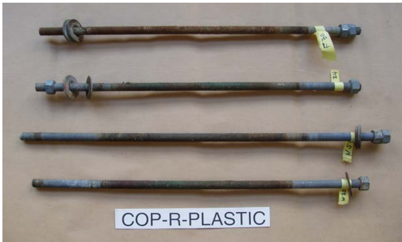
Figure II-1. Condition of Cop-R-Plastic coated galvanized threaded rods after six years exposure in Douglas-fir pentachlorophenol treated pole stubs.
