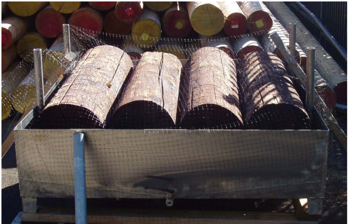
Figure VI-1 (cont.). Photo showing the two six-pole configurations a) configuration 1, b) configuration 2, and c) the four-pole configuration evaluated in our small scale preservative migration chamber.
