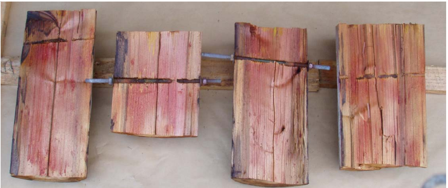
Figure II-2 Degree of a) copper [blue color] and b) fluoride [yellow color] movement away from the sites in Douglas-fir poles where Cop-R-Plastic coated galvanized rods were installed four years earlier.
