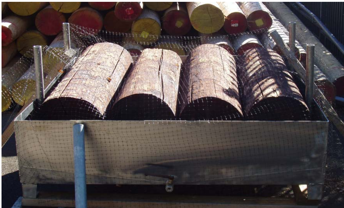
Figure VI-1 (cont.). Photo showing the two 6 pole configurations a.) configuration 1, b.) configuration 2, and c.) the 4 pole configuration evaluated in our small scale preservative migration chamber.
