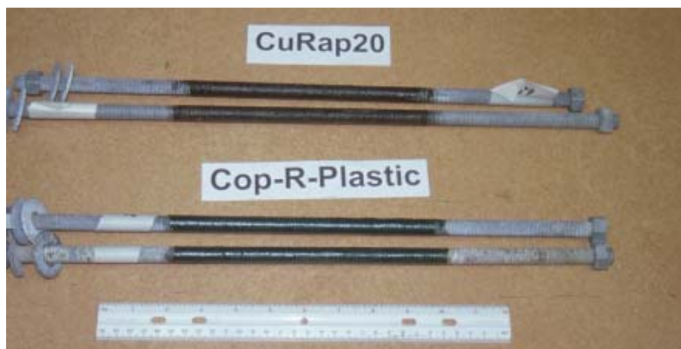
Figure II-1. Examples of galvanized rods coated with copper/boron (CuRap20) and copper/fluoride (Cop-R-Plastic) pastes.
