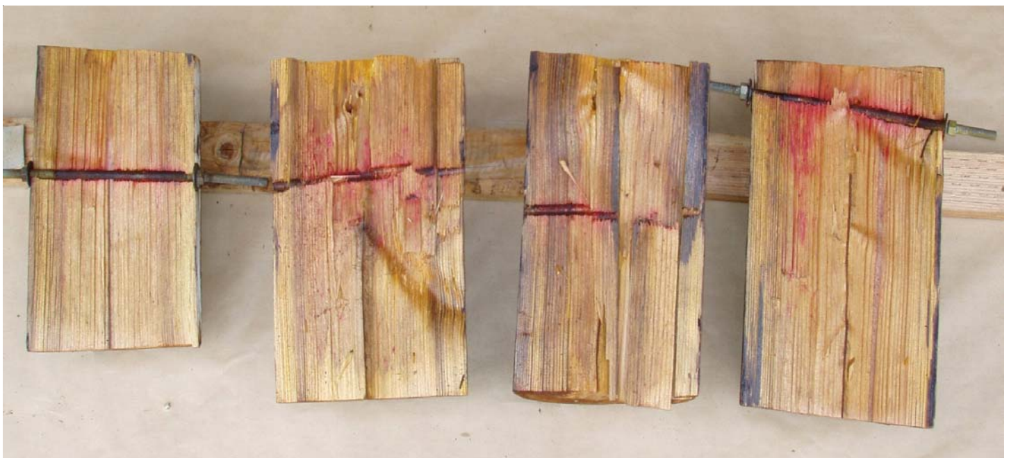
Figure II-3 Degree of a) copper [blue color] and b) boron [red color] movement away from the sites in Douglas-fir poles where CuRap 20 coated galvanized rods were installed four years earlier.
