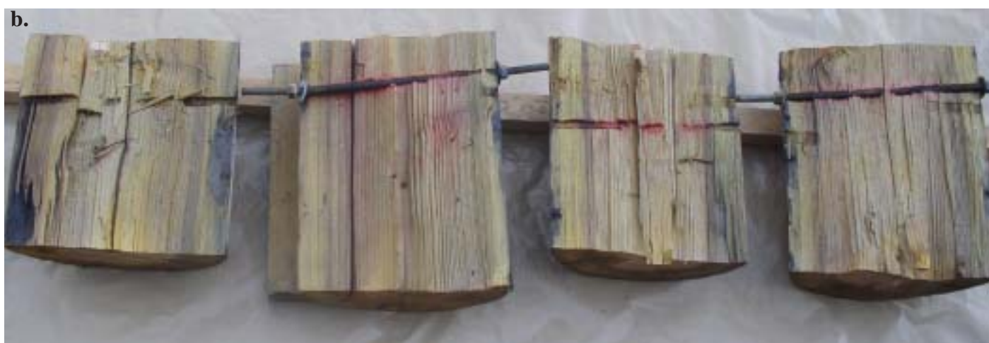
Figure II-3 Degree of a) copper [blue color] and b) boron [red color] movement away from the sites in Douglas-fir poles where CuRap 20 coated galvanized rods were installed three years earlier.
