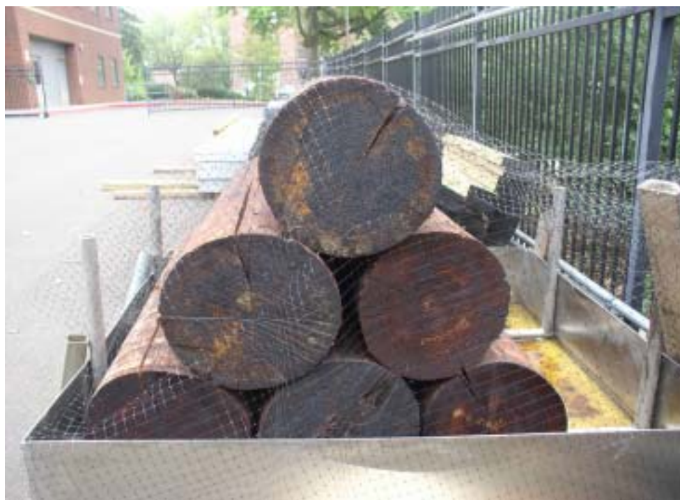
Figure VI-1. Photo showing the two 6 pole configurations a)configuration 1 and b) configuration 2 evaluated in our small scale preservative migration chamber.
