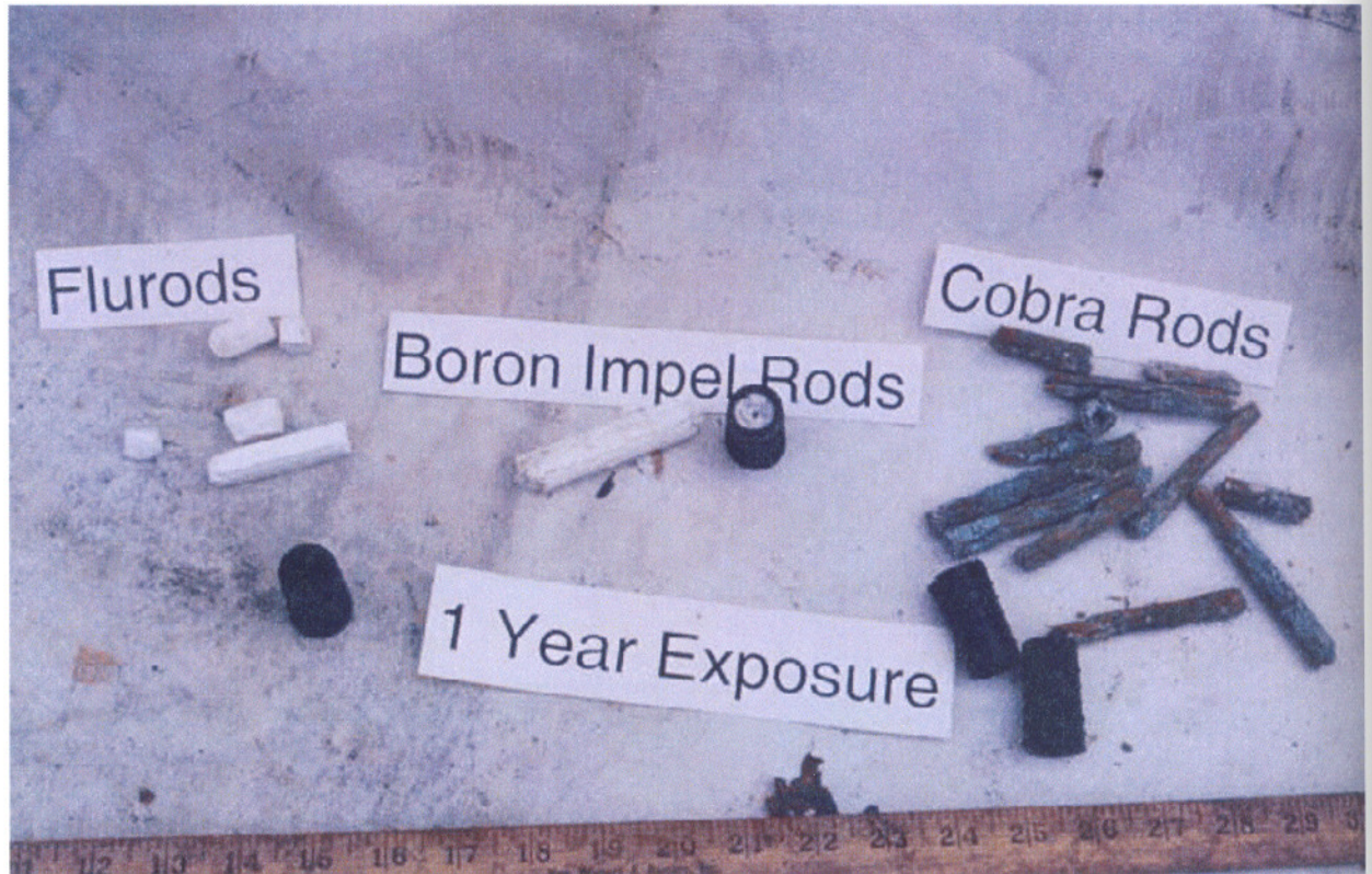
Figure I-17 Condition of fluoride, fused borate, and copper/borate rods removed from poles one year after application.
