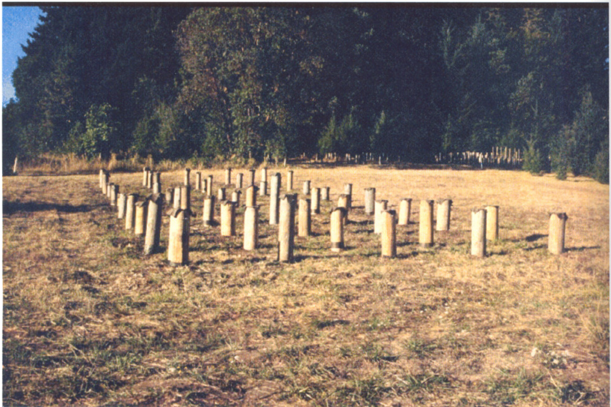
Figure IV-5 Douglas-fir poles at the Corvallis test site treated with selected external preservative systems.
