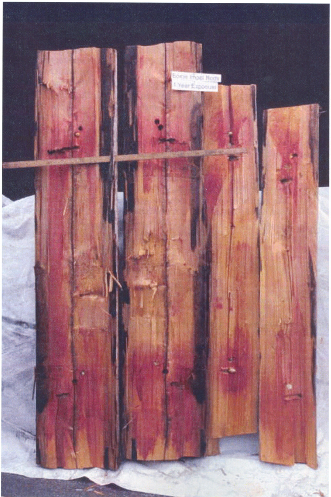
Figure I-15 Degree of boron movement in Douglas-fir pole sections treated with fused borate rods in three holes drilled around the pole at two locations one meter apart as determined using an indicator which turns red in the presence of boron.
