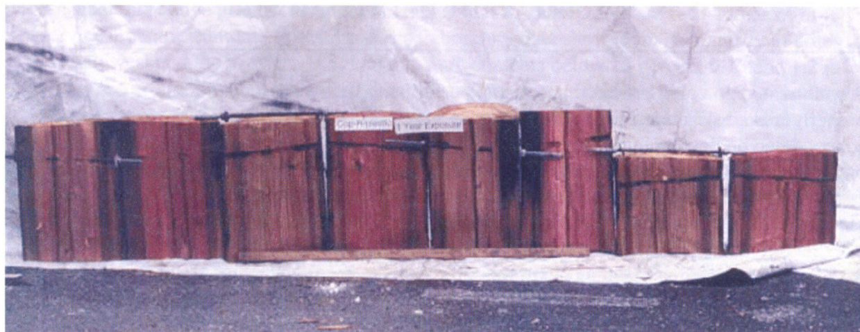
Figure II-3 Degree of copper and boron movement away from the sites in Douglas-fir poles where CuRap 20 coated galvanized rods were installed one year earlier.
