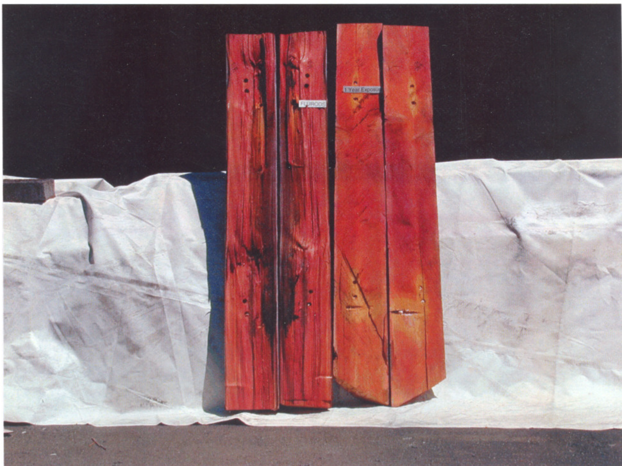
Figure I-14 Degree of fluoride movement in Douglas-fir pole sections treated with fluoride rods in three holes drilled around the pole at two locations one meter apart as determined using an indicator which turns yellow in the presence of fluoride.
