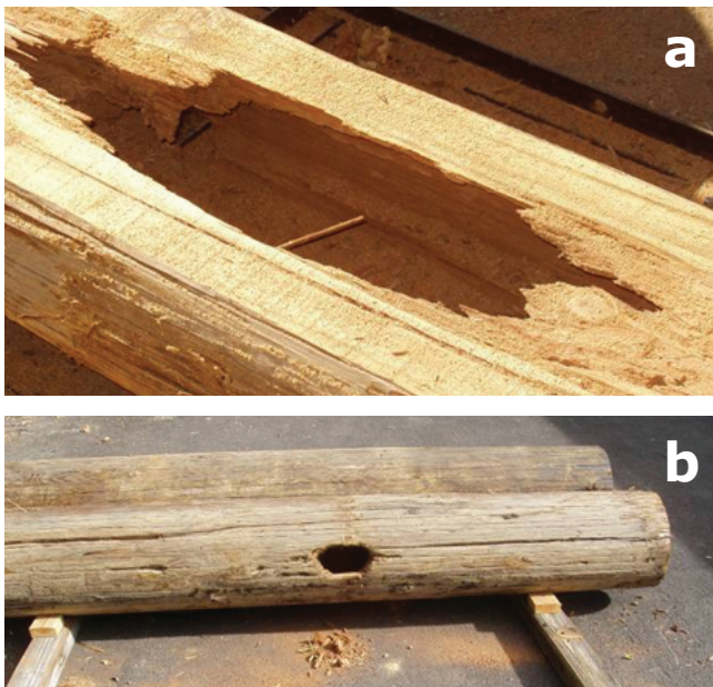
Figure 24. (a) Example of a woodpecker hole on the pole surface and (b) the extent of void associated with a nest.
