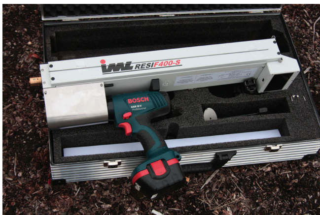
Figure 39. The resistograph drill uses a very fine bit to detect voids or softer wood that may be decayed.
