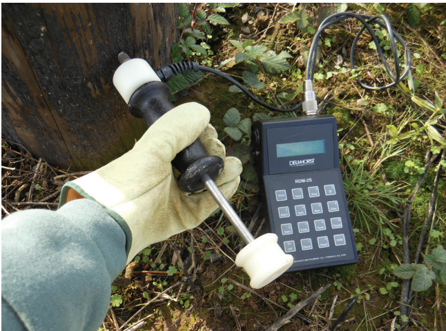
Figure 38. A resistance-type meter can be useful for detecting MC levels that are high enough (over 20%) for decay. As a sliding hammer drives two electrodes into the wood, a ruler emerging from the top of the hammer measures their depth. Shanks of the electrodes are coated so moisture readings are made between the uninsulated points.
