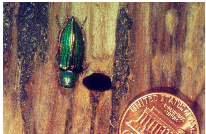
Figure 23. Golden buprestid beetle ( Buprestis aurulenta ). As an indication of internal rot in the aboveground portion of poles, look for the oval holes (0.5 in. long), that the buprestid beetle leaves as it emerges from wood. Many holes could mean an unsafe pole.
