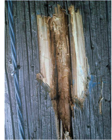
Figure 14. Weathering of a cedar pole turns the surface grey, but the wood underneath is unaffected.
