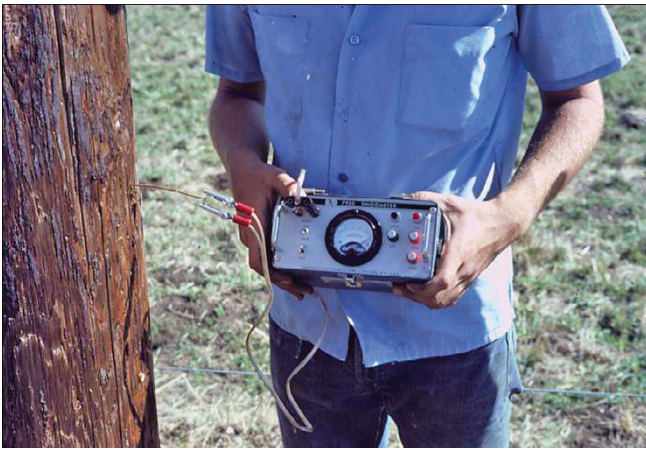
Figure 37. The Shigometer™ measures electrical resistance to detect rot in poles. Use an increment borer to determine the nature of the defect.
