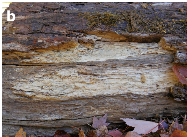
Figure 18. (a) Brown, (b) white, and (c) soft rot.
