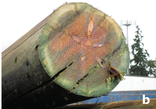
Figure 5. Incising and through-boring can markedly improve preservative penetration. (a) Cross section of a deep-incised pole and (b) a copper naphthenate through-bored pole.
