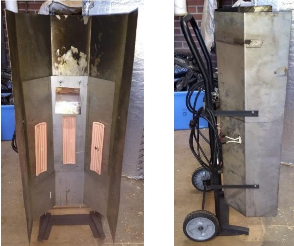
Figure 3.2.1: Modified fire ceramic panel-based testing apparatus made in 2020 in face view and profile.
