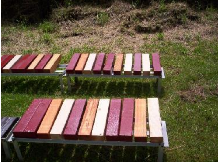
Figure 3.1.6: Polyurea coated and non-coated samples shortly after exposure in Hilo Hawaii. After 4 years of exposure the non-treated, non-coated Douglas-fir samples began to experience decay on the sides and undersides where moisture collected and there was evidence of fungal fruiting bodies in the untreated samples (Figure 3.1.7). These samples had an average rating of 7.0 on a scale of 10 (perfectly sound, no evidence of biological attack) to 0 (complete failure). Non-coated penta treated samples had some weathering on the upper surfaces, but remained sound and free of decay. All of the penta treated, non-coated samples rated 10.
