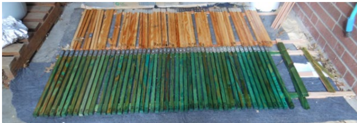
Figure 3.3.1. Stakes drying under cover after treatment with copper naphthenate (bottom) or penta (top).
