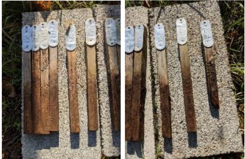
Figure 3.3.7: Stakes rated at the 70-month sampling. Stakes that failed in 2020, predominantly due to brown-rot (top left).
