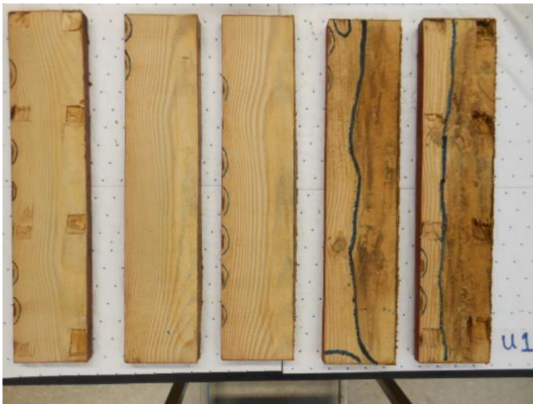
Figure 3.1.10. Interior of a coated, untreated Douglas-fir section after 6 years of aboveground exposure in Hilo, Hawaii.
