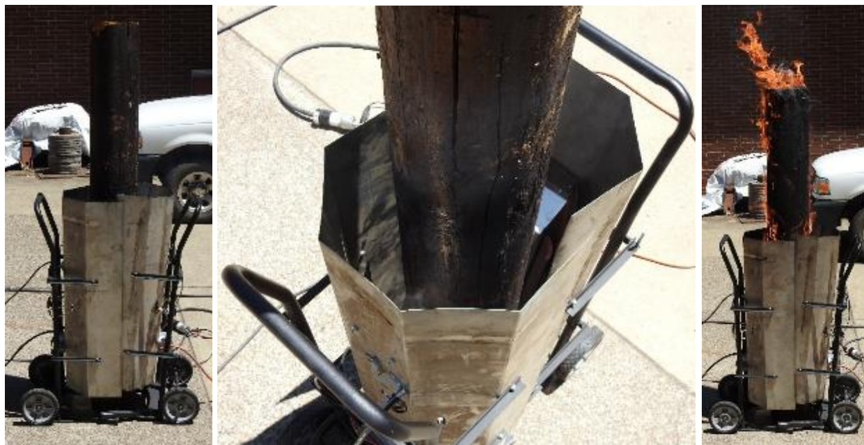
Figure 3.2.2: Orientation of two identical burn units during a fire test at different stages, during heating and then after combustion.
