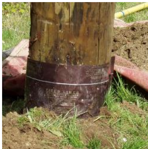
Figure 4.1.1: Example of a Biotrans liner at the OSU Peavy Arboretum test site.
