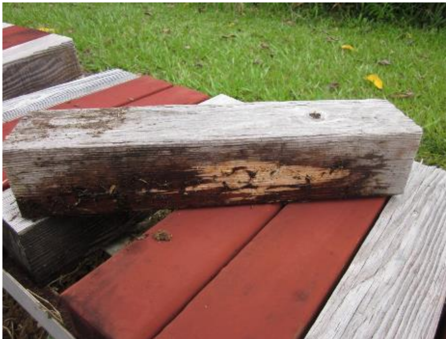
Figure 3.1.7. Example of a non-treated, non-coated wood sample after 4 years of exposure in Hilo, Hawaii, showing evidence of fungal decay and fruiting bodies
