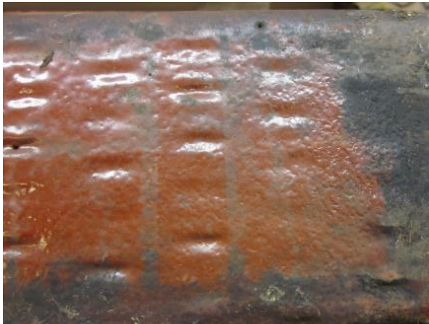
Figure 3.1.8. Example of lower, non-UV exposed surface of a coated, penta treated section showing evidence of oil migration towards the surface after 6 years of exposure in Hilo, Hawaii
