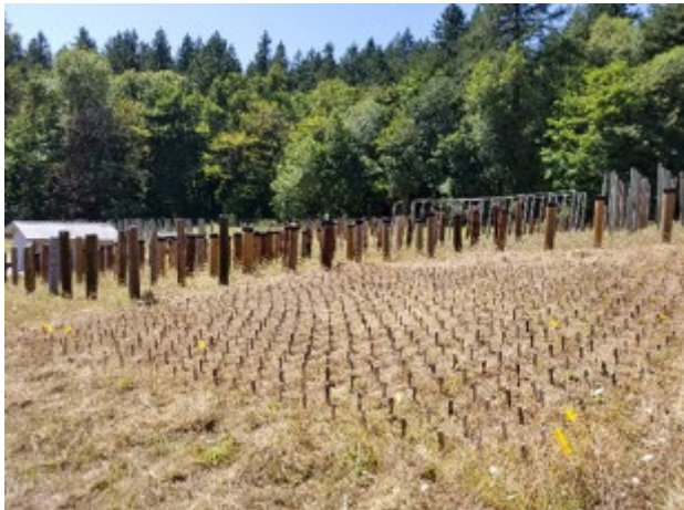
Figure 3.3.5: Average ratings of stakes treated with pentachlorophenol using biodiesel and diesel-containing solvents for 70 months at an open field site.
