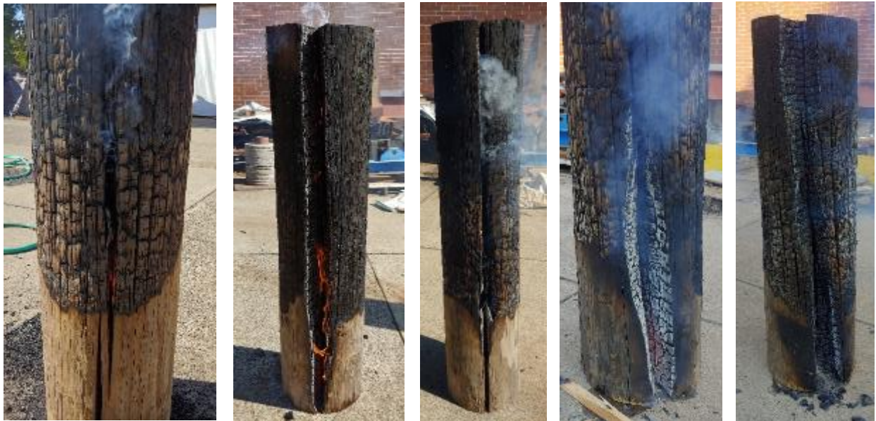
Figure 3.2.3: Examples of untreated poles with checks smoldering. Checks acted like chimneys and extended caused vigorous smoldering during the smoldering period.
