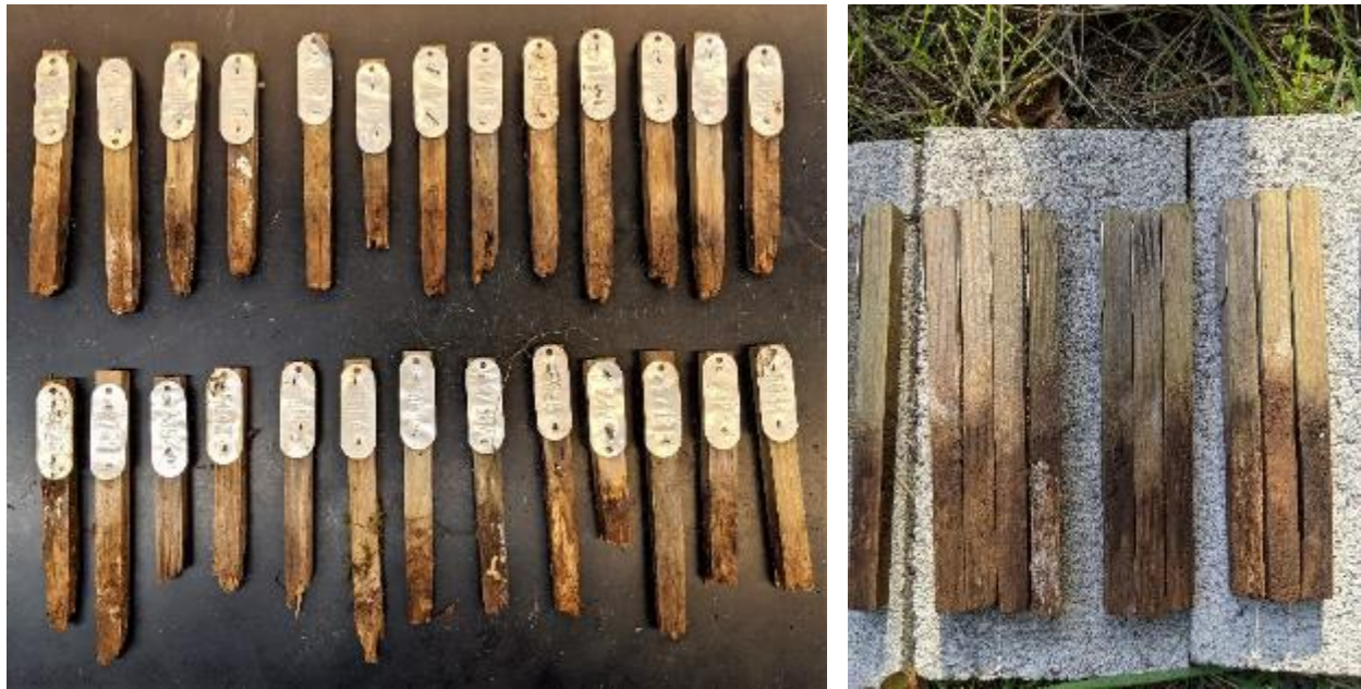
Figure 3.3.7: Stakes rated at the 70-month sampling. Stakes that failed in 2020, predominantly due to brown-rot (top left).
