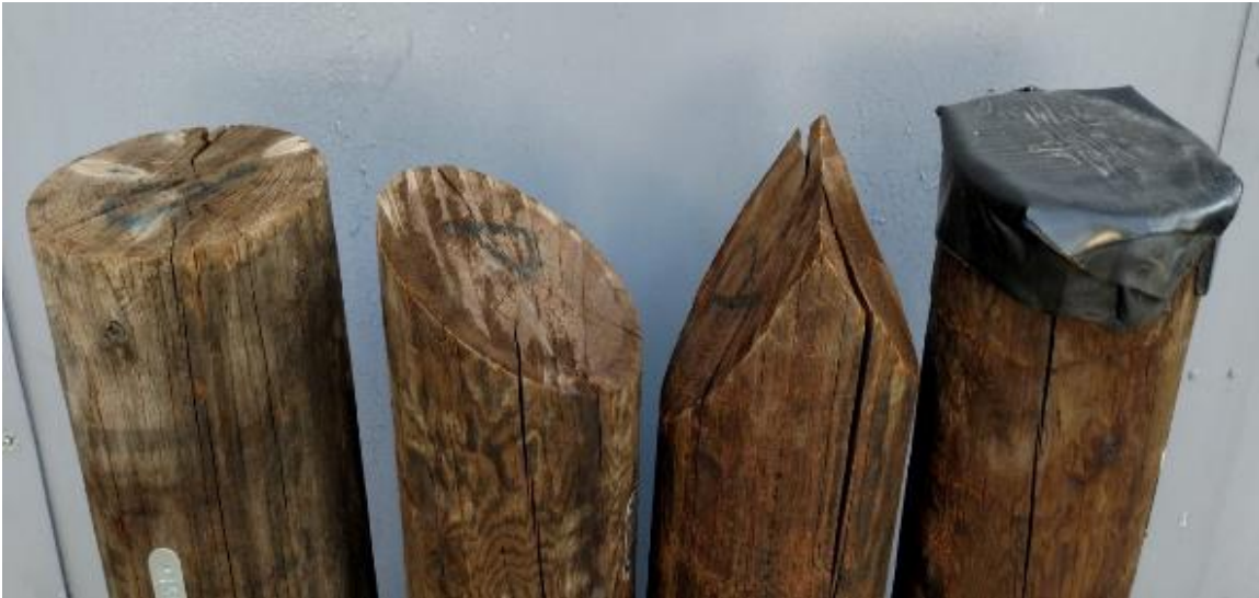
Figure 3.1.4. Examples of the different pole top roofing patterns assessed for their ability to resist moisture ingress.
