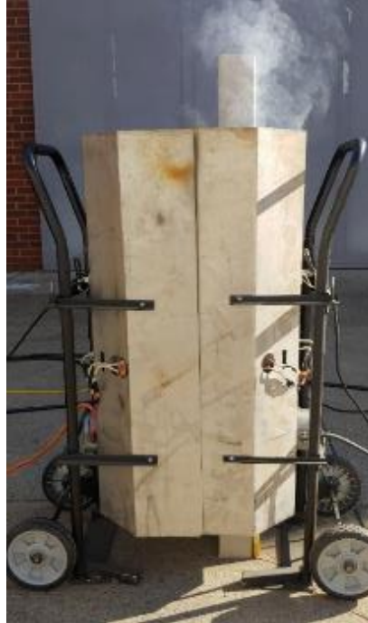
Figure 3.2.6: Fire testing apparatus adapted to testing crossarms and fire-retardant treatments for crossarms. Two racks were used to enclose the space around the test crossarm. The crossarm was placed close to one of the heating elements and the burn was initiated.
